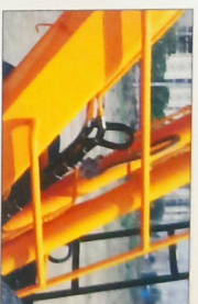
Cylinder with O.C. Valve Lift Cylinder with O.C. Valve for Protection of Hydraulic Handling of Load.
