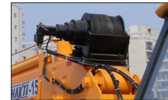
Winch Heavy Duty Big Drum Double Bearing Winch for Precision handling with 6 Fall Hook Block.
