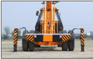
Outriggers Extendable Outriggers for Extra Stability.
